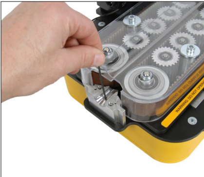
Loosen and remove the M2.5 screw securing the guide into the housing
